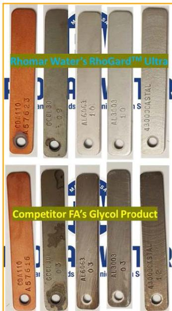
**FIGURE 2:** These images are for aluminium (AL6063, AL3003, 4300CASTAL), copper (CDA110) and cast iron (GCCL30) coupons after procedural cleaning, drying and weighing according to the ASTM standards.
